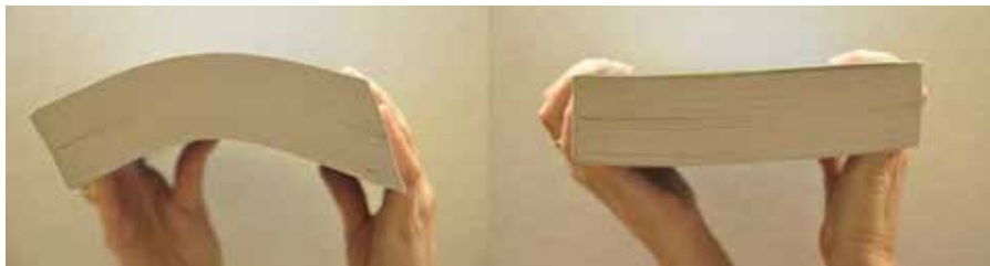
Figure 3.3: A paper book before and after its pages has been glued together
